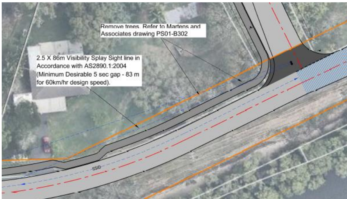
Figure 3.3 Site Access Arrangements
