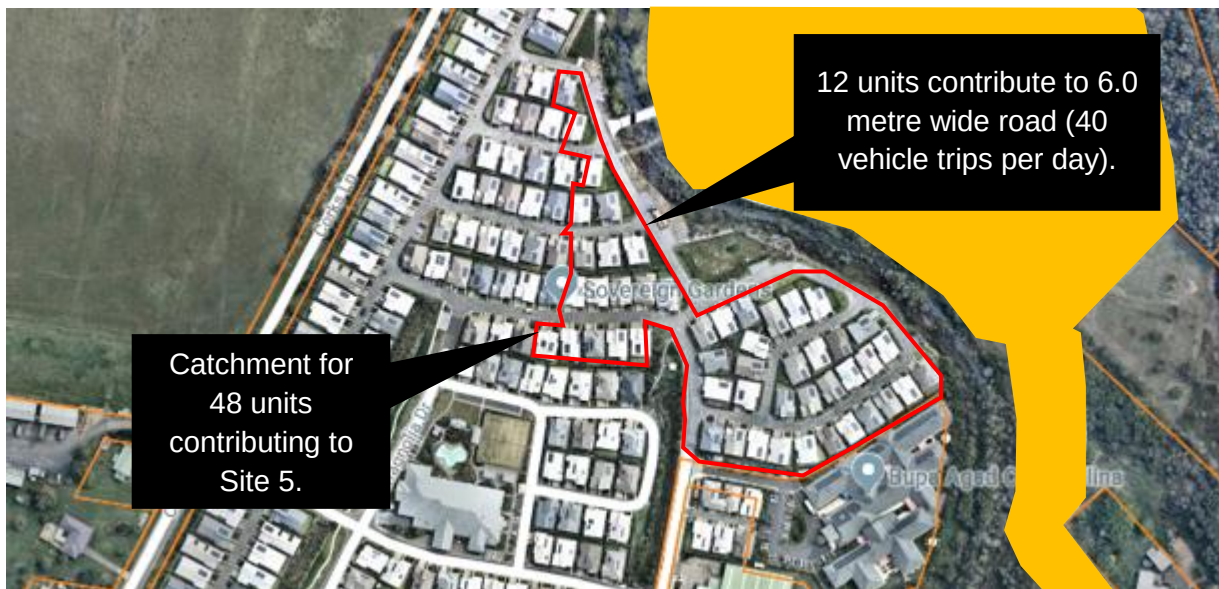
Figure 6.8 Bupa Entry Road Vehicle Catchment
